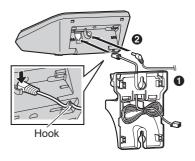
3 Insert the hooks on the wall mounting adaptor into the holes (A) and (B) on the base unit.
